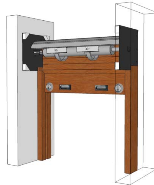
Between Wall Mount Without Lintel
