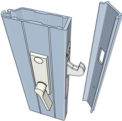
Dry fit the Interlocking Jamb Molding against the wall, directly under the track. It should fit snugly against the wall and the track at the top. If it needs to be trimmed, trim it at the **BOTTOM**. The arrow sticker on the back pointing up can easily determine top and bottom. The latch slot should correspond to the hook of the latch.
