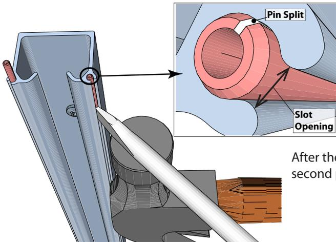
After the track has been secured, drive the alignment pins back halfway into the second piece of track with a hammer and the edge of a screwdriver.
