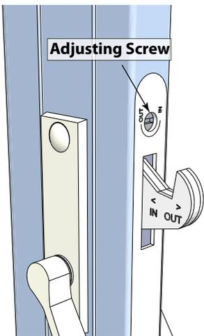
Shut the door, latch it and wiggle the handle a bit. The Latch should swing fully up with the Lead Post pulled snugly against the Interlocking Jamb Molding.
