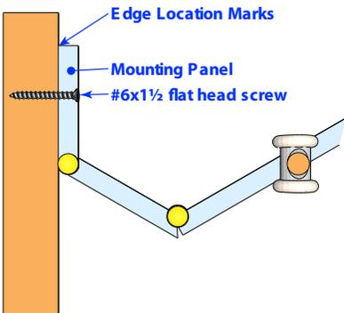
Insert #6 x 1 1/2" flat head screws about 8" up from the floor and 8" down from the track.
