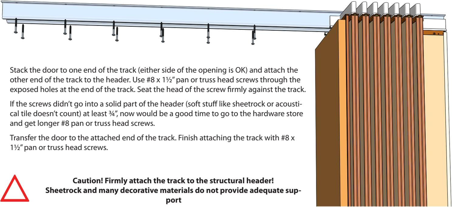
Stack the door to one end of the track (either side of the opening is OK) and attach the other end of the track to the header. Use #8 x 1½" pan or truss head screws through the exposed holes at the end of the track. Seat the head of the screw firmly against the track.
