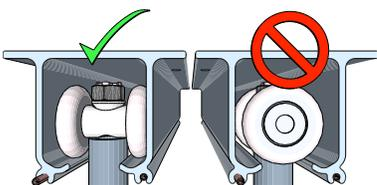
Thread the track onto wheels; lineup the wheels properly in the track grooves. Be careful not to insert the wheels sideways. You won't like the result.
