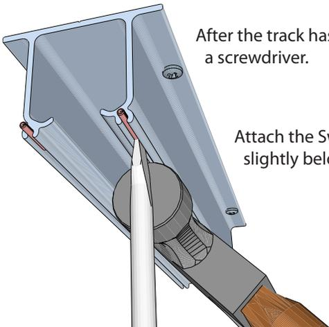
After the track has been secured, drive the alignment pins across the joints with a hammer and the edge of a screwdriver.
