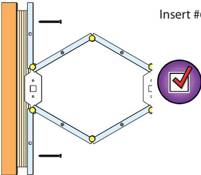
Insert #6 x 1½” flat head screws about 8” up from the floor and 8” down from the track on both sides.
