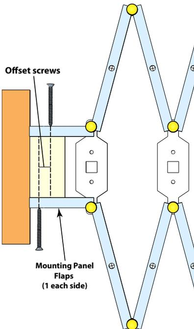
Push the door over the post. The post will snugly fit between the mounting panel flaps. Screw the mounting panel flaps to the post using the provided #6 x 1½ flat head screws. Place a screw about 6" from the top and bottom of the post and 2 additional screws equal distances between the first 2 screws. Repeat anchoring the 2nd flap being sure to slightly offset the screws so they won't meet in the middle of the post.
