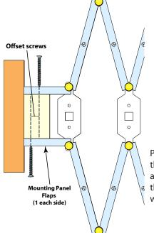
Push the door over the post. The post will snugly fit between the mounting panel flaps. Screw the mounting panel flaps to the post using the provided #6 x  $1\frac{1}{2}$  flat head screws. Place a screw about 6" from the top and bottom of the post and 2 additional screws equal distances between the first 2 screws. Repeat anchoring the 2nd flap being sure to slightly offset the screws so they won't meet in the middle of the post.
