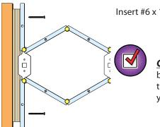
Insert #6 x 11/2" flat head screws about 8" up from the floor and 8" down from the track on both sides.
