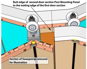
Drive the #6 x 1½" screws through the pre-drilled holes in the Post Mounting Panels into the post.
