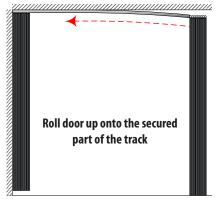
Stack the door to one end of the track (either side of the opening is OK) and attach the other end of the track to the header. Use #8 1½" Pan head screws to attach the track to the header and put in enough screws to accommodate the stacked door. Seat the heads of the screws firmly against the track.
