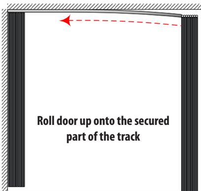
Roll door up onto the secured part of the track
