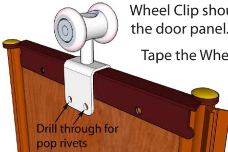
Tape the Wheel Clip in place using painters masking tape.
