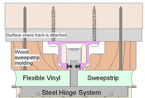
Use the 8d (2 1/2") finishing nails, approximately 1 per foot, to attach the wood Sweepstrip Moldings tightly against each side of the track.
