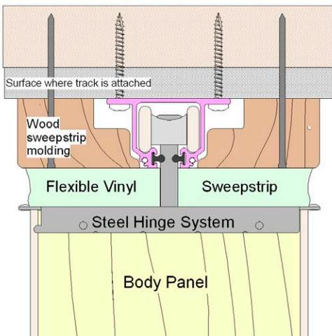
Use a flat bladed prying tool to remove the sweep strips on both sides of the track.
