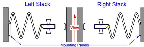
Remove the #6 x 1 1/2" Flat head screws securing the mounting panel to the jam. Stack the door back against the mounting panel and door jam.
